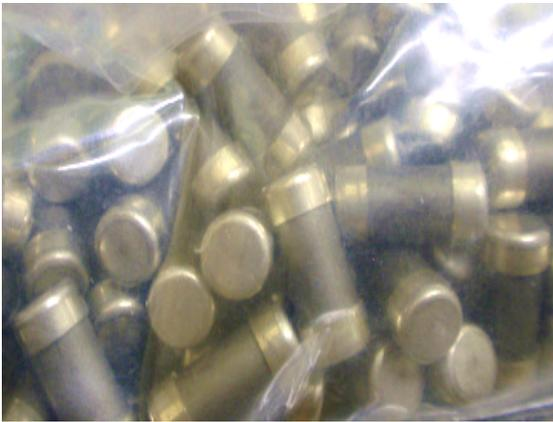
Close up of the silver end caps connected to the "cut" resistor body, with its dark grey/black Tantalum resistive coating ready to go into the machine that puts the solid silver lead out wires on the body, we had to invest in a completely new spot welding apparatus as the one used to connect the tinned copper wire to the standard nickel – iron and high copper brass end caps was so hot it melted the silver wire so it just fell off instead of being connected to the end cap.
