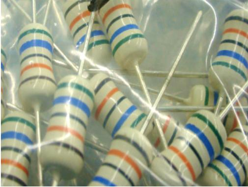
Voila!, the world's first "mass produced" Tantalum silver capped and wired resistors, well perhaps mass produced is a bit rich, as we only made 9,600 pcs between 48 values, but still.
