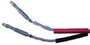
PIC 3 ends before heatshrink fitted
