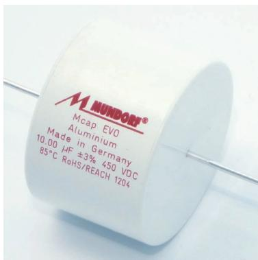
The **MCap® EVO** was designed in 2012 as the successor of the RXF to facilitate utmost musical enjoyment even in small spaces on a limited budget. The PP capacitor film used here is first metallised with the thickest possible aluminium layer, then wound precisely into innovative EVO-LUTION winding geometry and then potted by hand into special casings.
