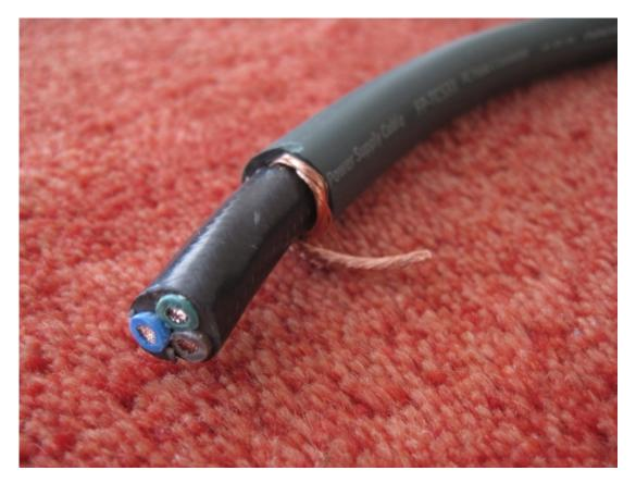
Above: FP-TCS31 cable with outer sleeve removed and screening mesh combined into a strand.
