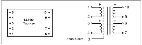
44 x 30 x 23 **Dimensions** (L x W x H above PCB, in mm) 5.08 mm (0.2") Spacing between pins 30.48 mm (1.2") Spacing between rows of pins Rec. PCB hole diameter: 1.5 mm 93 g Weight: Static resistance of each primary:  $1.2 \Omega$  $6.4~\Omega$ Static resistance of each secondary:
