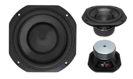
The SB2201 has been optimised for bass performance in sub-woofer applications. It uses a vented, symmetrical field magnet system with an exceptionally long voice coil for large linear excursion capability. The cone uses a long fibred pulp for rigidity and with the dustcap, is damped by a coat of glossy black dope. Suspension stiffness and excursion is optimised for tight control over high power transients
