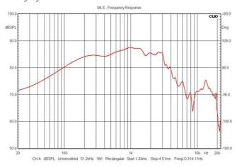
Frequency response from driver in small cab with front baffle dimensions 190 x 300 mm. Smooth roll-off characteristic provides easy filtering.
