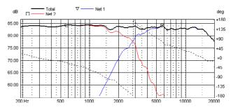
Example of two-way set-up with JA-2806 tweeter in 7- litre monitor.
