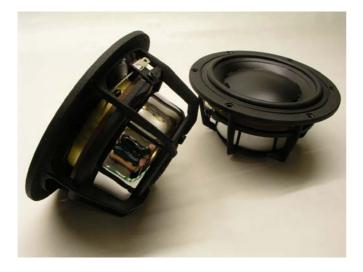
The JA-5004 provides a powerful 5" midbass driver fitted with a polypropylene cone and a massive 75 mm voice coil ensuring high power handling. A thoroughly vented spider chassis provides free air ventilation and absence of compression. The driver may be used in small 2-way monitors or as midrange driver in larger 3-way systems.
