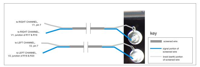
Rear view of 300BSEp with phono sockets and insulation plugs fitted
