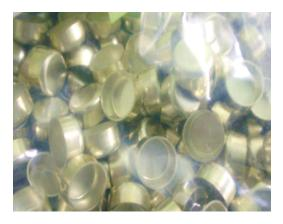
The punched end caps after selection, we have to hand select end caps as many end caps are deformed and cannot be used.
