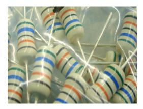
Voila!, the world's first "mass produced" Tantalum silver capped and wired resistors, well perhaps mass produced is a bit rich, as we only made 9,600 pcs between 48 values, but still.
