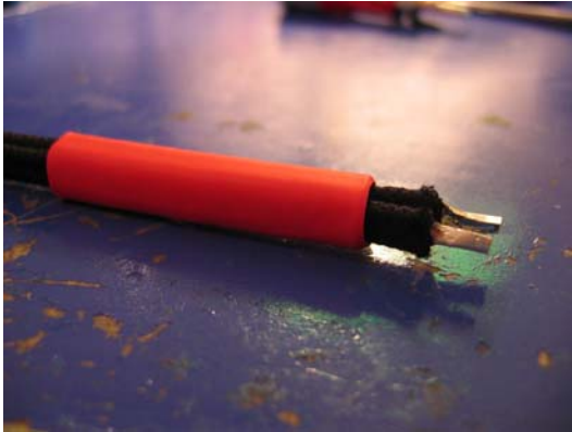
Figure 3 Heat shrink is applied as with Duelund 2.0 shown here
