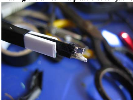
Figure 6 Two Duelund 0.5 wires side-by-side sandwiched between white plastic strips ready for application of heat shrink sleeve
