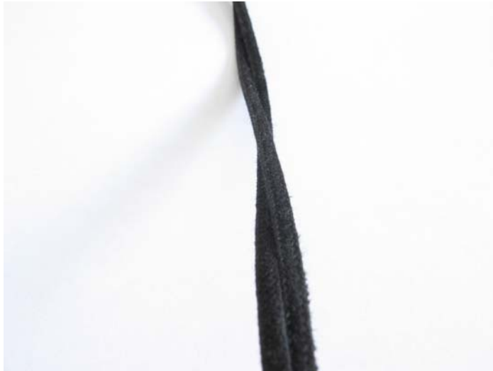
Figure 5 Wires passed across each other, flattened surfaces uppermost
