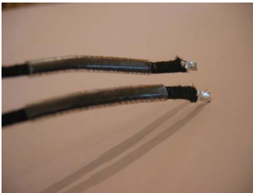
Figure 2 Clear heat shrink applied
