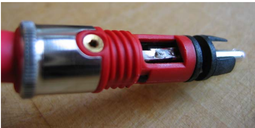
Figure 4 WBT Silver Plug with Duelund 0.2 wire soldered in place
