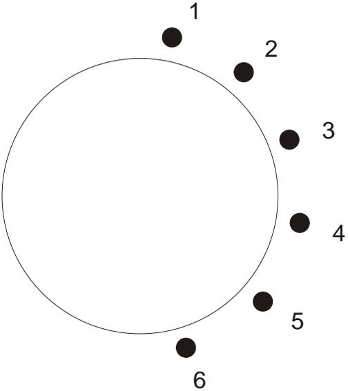
To change to a 2 pole/2 way/3 way/4 way/5 way, screw the locator screw into the correct numbered hole on the front of the selector switch
