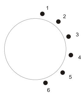
To change to a 2 pole/2 way/3 way/4 way/5 way, screw the locator screw into the correct numbered hole on the front of the selector switch
