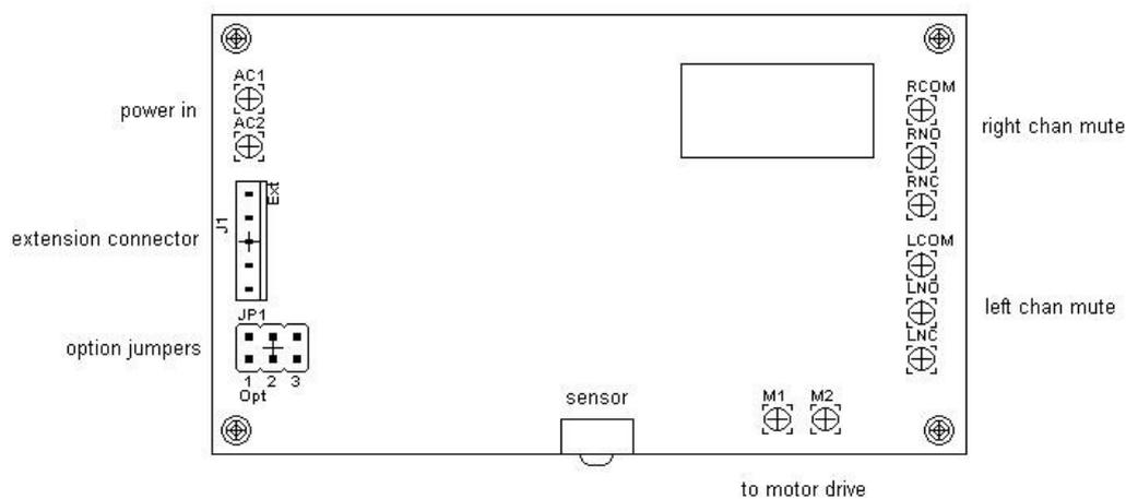
The board is designed to be powered by 6.3V (standard heater supply) to 15V AC supply or a DC supply ranging from 6.3V to 15V DC. The polarity of the supply is not important.
