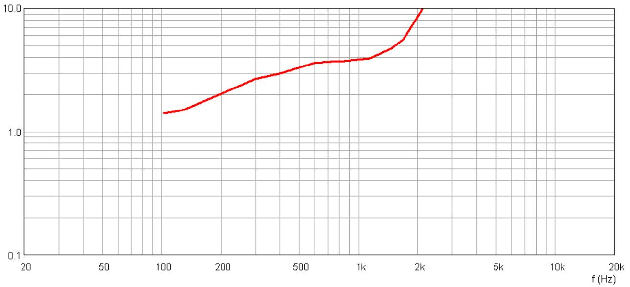
**The curve maximum RMS voltage at low frequencies.**
