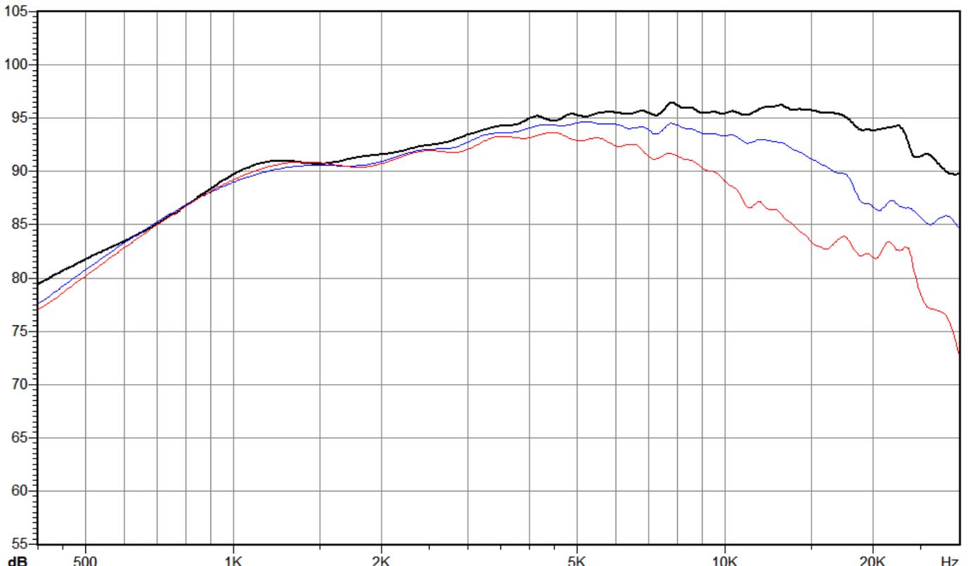
Frequency responses measured at angles of 0, 30, 60 degrees to horizontal
