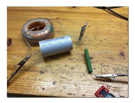
Then you do the impedance measurement, i.e. 100-5000 Hz, depending on the capacitors value (in this example a 5.6 uF was used).
