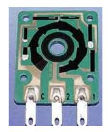
In case of the Ladder circuit, they are supposed only to be used for dividers or volume controls, but not for variable resistors.
