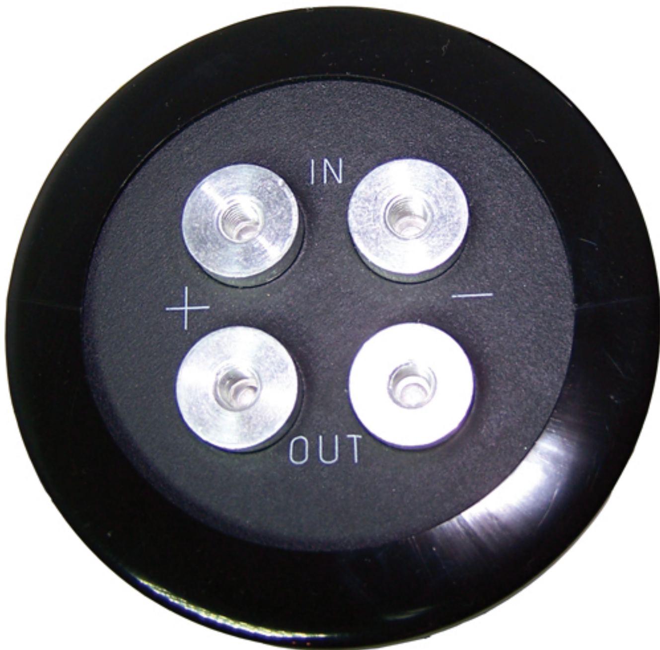
Top View of capacitor, note well, some values do not show "IN" or "OUT" however the orientation is the same
